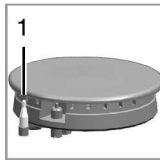
1. Gas shut off safety
