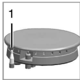
1. Gas shut off safety
