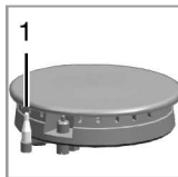
1. Gas shut off safety
