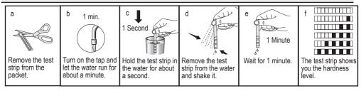
After determining hardness level of the supply water:
