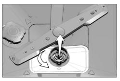
2. Pull out the metal/plastic filter (3) from the seating.
