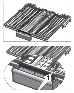
In models with partial movement feature, pushing the bar (1) on the handle enables the central tray of the basket to get to the lower position and the system gets unlocked. Thus right and left side trays can be used as moving parts.
