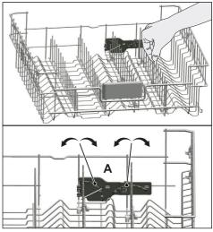
Bringing the tines to the horizontal position by holding them from the tips may cause them to bend. Therefore, it will be appropriate to bring the tines in the middle to horizontal or vertical position by holding them from their stems and pushing in the direction of arrow.
