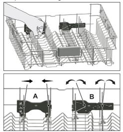
Holding the tines from ends to put them in lying position may cause the tines to bend. For this reason, it will be appropriate to hold the tines in the middle from their bottoms and to push in the direction of the arrow to lay down or bring them to vertical position.
