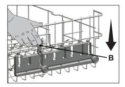
Repeat the same process to lower the other side of the basket. Make sure that both sides of the loaded basket height adjustment mechanism are at the same level (down or up).
