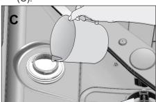
4. Fill the salt reservoir with salt by using the salt funnel (D). To speed up dissolution rate of salt in water, stir it with a spoon.
